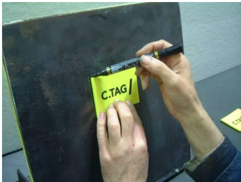
1. Marking out around the marker, ready for masking off the area to be bonded.
