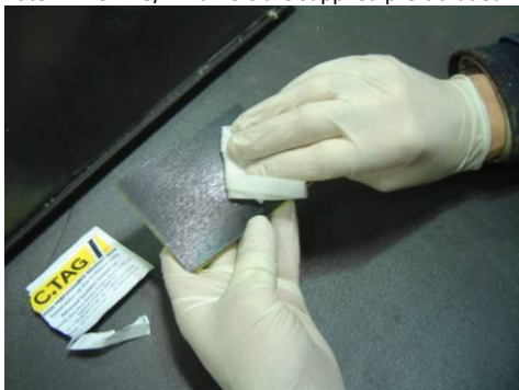
5. De-grease the back of the C.TAG/® to be bonded
