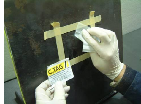
4. De-grease substrate surface to be bonded
