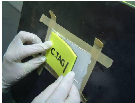
10. Check marker orientation; align the C.TAG/® with an edge tape, leaving a 1-2 mm gap.....
