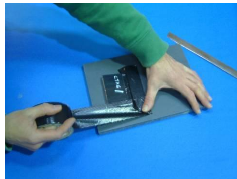
16. After checking the marker has bonded correctly, and final cleaning of the marker face, the cover is taped in place until the structure is ready for deployment.
